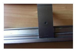
**Step 4**: Tighten screw on bracket
