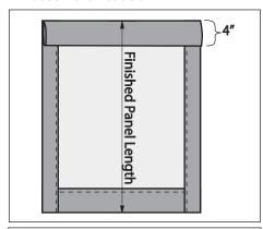
2. Measure the panel width. Cut a strip of Serpentine tape 2 times the panel width, plus 20" extra.
