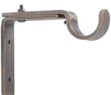
Adjustable Single Bracket POBKT118 1" W x 3 1/4" H backplate, adjustable 3 1/2" - 5" return Metal, Luminous
